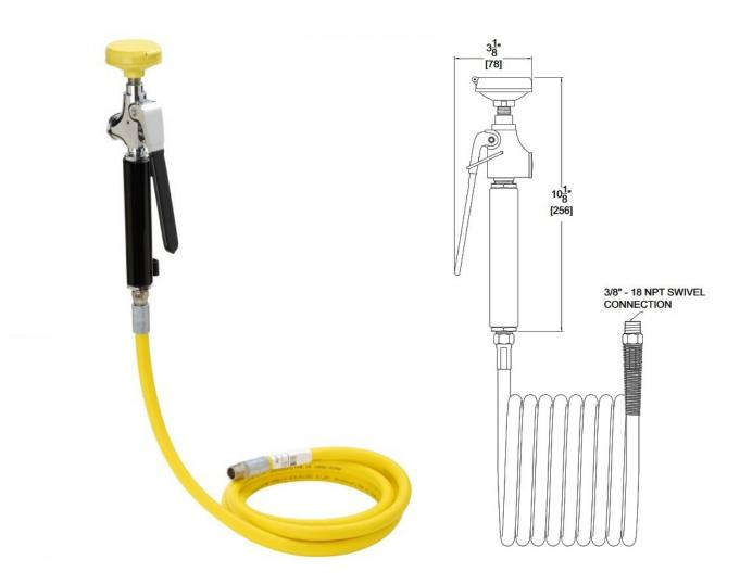
Model S0002 is our unmounted eye/face and body drench hose, complete with yellow plastic spray head, stay open squeeze lever valve and 2.4m long reinforced PVC hose.
